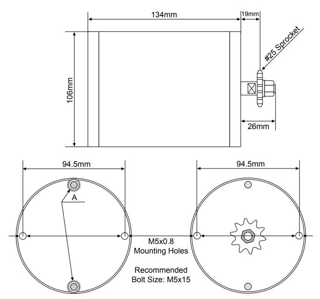
A = Recessed motor assembly bolts provide a flat backplate with no bolt heads protruding out of it.
