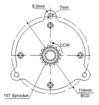
This motor can only be used with its shaft spinning counterclockwise. If wired to spin clockwise the sprocket will not engage.
