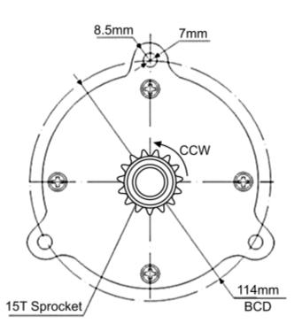
This motor can only be used with its shaft spinning counterclockwise. If wired to spin clockwise the sprocket will not engage.
