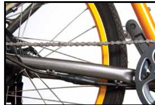
E3Metro, showing quick disconnect plug on chain stay.
