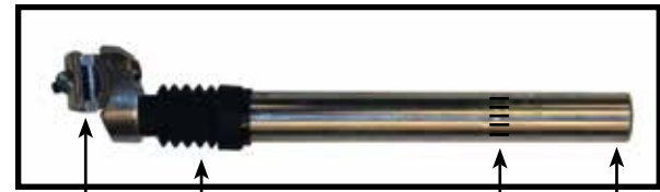
Attach Seat Here, Boot, Minimum Insertion Mark, Preload adjusting screw on underside
