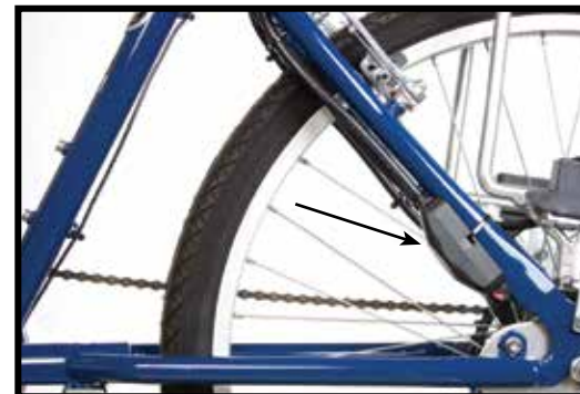
Via Lento, showing quick-disconnect box on seat stay.
