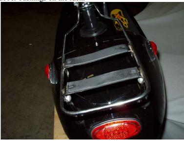
Then place the trunk on the rack over the rubber bushings. The two metal plates are placed inside the trunk and secured to the rack with the four enclosed screws and nuts.
