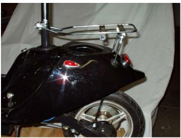
Attach the optional trunk to the trunk rack. Your trunk comes with the necessary hardware to attach the trunk to the rack if you choose. In the picture below are 2 rubber bushings and metal plates along with 4 screws and nuts.
