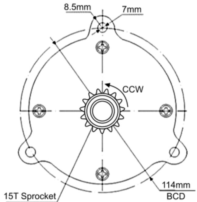
This motor can only be used with its shaft
