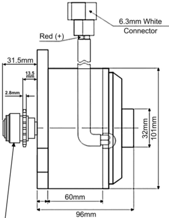
15T Sprocket with One-Way
