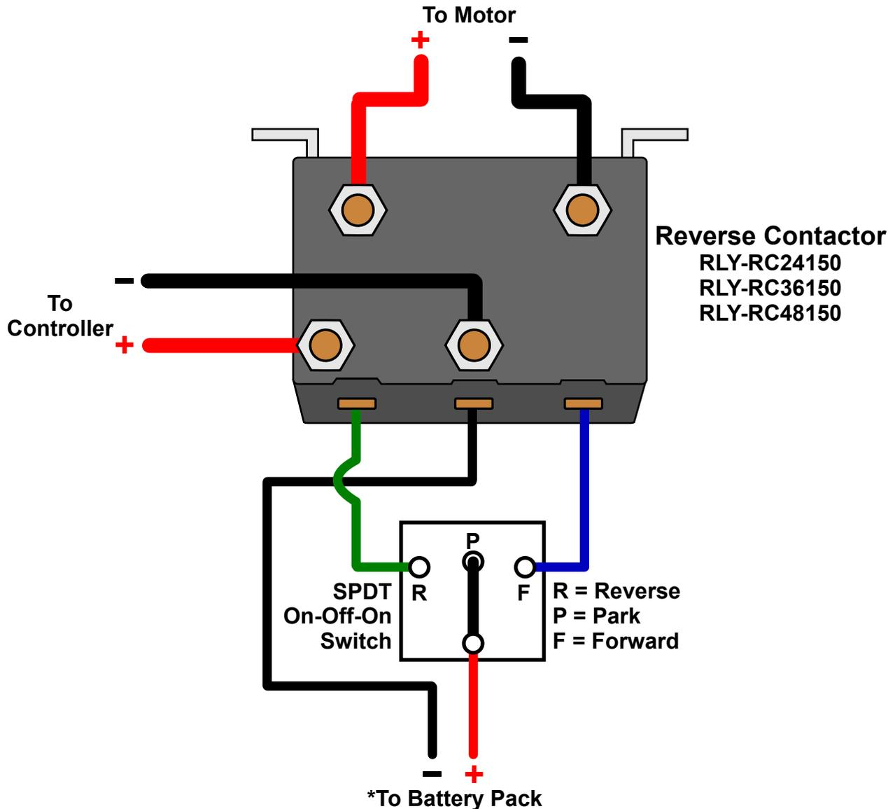
\*A pole of the main power switch or a relay that is activated by the main power switch should be wired between the battery pack and reverse contactor so the reverse contactor's coil will not remain energized if its switch is left in the forward or reverse positions while the vehicle is not being used.
