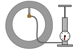
6- Insert valve stem through hole in rim.7- Push tire and tube over so the tube is inside the rim.
