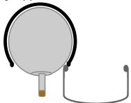
**9**- Starting at the valve stem, carefully push the second tire bead into the rim using only your hands.
