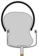
**10**- Push the valve stem base up into the tire so it is not caught between the tire beads and the rim.
