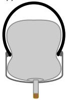
**12-** Deflate the tire. This will help avoid pinching the tube when the tire is inflated to full pressure.
