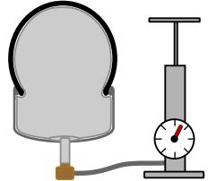
**2**- If bubbles appear in tub of water that tube is submersed into replace faulty tube with new tube and retest. If no bubbles appear in tub of water remove and partially deflate tube.
