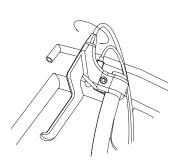
1 To adjust the brake, thread the adjuster in or out 1/4 to 1/2 turns until the desired brake adjustment is attained.
