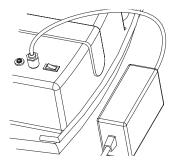
**1** Plug the charger into the port on the Ground Force Drifter. Make sure the power switch is in the "OFF" position.
