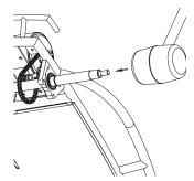
**5** Lightly tap the end of the axle with a rubber mallet. DO NOT USE A HAMMER as this will damage the thread. The brake drum and pulley must be slid along the axle as your tapping progresses.
