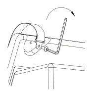
2 Install the shoulder belt anchor to the back of the seat. Insert and tighten securely.
