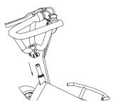
1 Untangle the wires and insert the steering wheel into the steering column.
