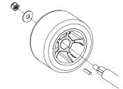
**1** To remove a wheel, remove the self-locking nut (13mm socket or wrench required for front wheels, 17mm for the rear wheels). Tap the wheel to remove.
