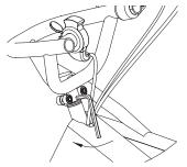
**2** Using a 5mm hexagonal wrench, tighten the steering wheel bolts to the steering column.
