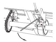
**2** Use a 3mm wrench to loosen the brake
