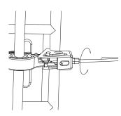
**2** If the adjuster is threaded outward and the brake still has too much slack, use the auxiliary adjuster at the rear brake for additional adjustments.
