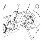
**4** Remove c-clips on the axle between the two bearings.
