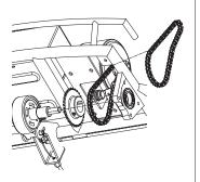
**6** When the axle end is clear of the bearing hanger, remove and replace the chain. Reverse this procedure to reassemble.
