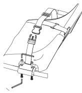
1 Position the seat over the frame and align it with the holes in the frame. Align the safety belt anchor holes to the holes in the seat and frame with the lap/shoulder assembly on the left and the receiver latch on the right. Insert the screws and tighten securely.
