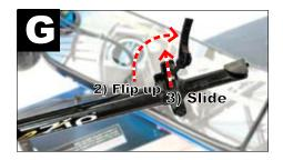
**8.** Raise the handlebar post, then close the hinge quick release by reversing step 6. If the quick-release lever feels loose or is not secure, its preload may need to be adjusted by tightening the 10mm preloadadjustment nut shown in photo **I**.
