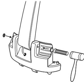
**11** Attach a fixed clip to both ends of the handle axle to secure the handle to the front board.
