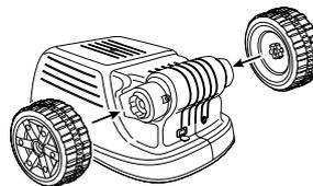
**3** Locate the 2 rear wheels (Rear wheels have gears on the inside). Slide one wheel over the axle until it interlocks with gearbox.
