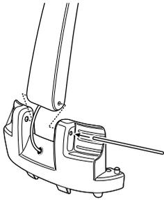
**10** Align holes on the handle with the holes on the front board and slide the handle axle through to the other side.
