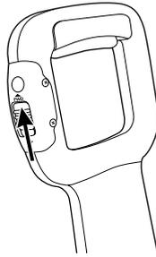
**2** Use the forward/reverse direction switch to select a forward or reverse motion.
