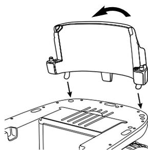
**15** To attach the rear board, lean board slightly forward, then pull back while pushing down until rear board is attached securely to the main body.
