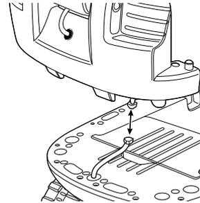
**12** Position the front board assembly to the body and connect the wires from the handle to the wires from the body.
