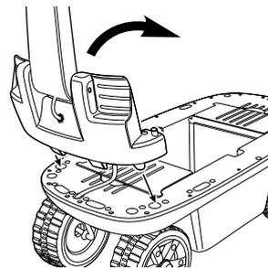
**14** Align the front board with the main body. Lean the front board slightly forward to hook the side pegs (See arrows), then pull back to the upright position while pushing down on the front board until it attaches securely into the main body.
