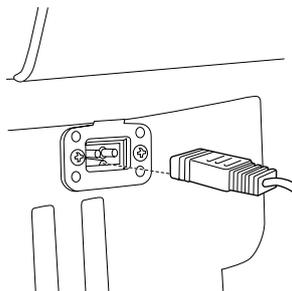
**1** Align the groove on the charger port with the corresponding tab on the Electric Wagon socket and insert into socket.
