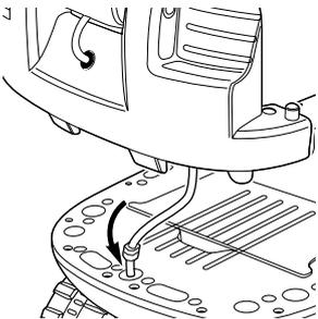
**13** Feed the excess wires into the opening on the main body.
