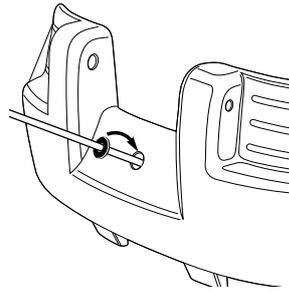
**9** Plug the hole on the front board with the rubber ring.
