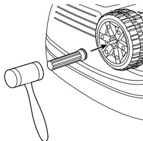
**5** Position the fixed clip and clip tool over the end of the axle. Using a rubber mallet/hammer, strike the tool to securely attach the clip onto the rear axle.
