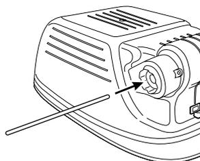
**2** Insert the rear axle into the hole in the gearbox and slide it through to the other side.
