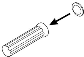
**4** Insert a fixed clip into the clip tool.
