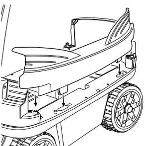
**16** Attach the left side board. Make sure side board is aligned properly with the front and rear boards before pushing down.
