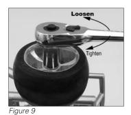
4B-2.) To replace a front wheel, make sure the bearings are seated and the center spacer is installed. Position the wheel so the Razor logo is toward the outside. Install the washer and tighten the self-locking nut securely. Refer to Figure 10 for assembly detail.
