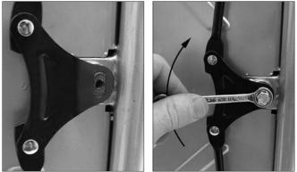
Figure 3a Figure 3b Tighten the tie-rod control arm using a 5 mm hex key wrench.
