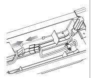
**6** Reconnect the motor connector, reinstall the cable clamping block (shown), and reposition the battery and replace cover, tighten cover screws.
