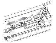
2 Using a Phillips screwdriver, remove the cable-clamping block and disconnect the motor connector from the controller.
