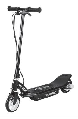
**NOTE:** The unit must be traveling at least 3 mph (5 kmh) before motor will engage. Kick start to at least 3 mph (5 kmh) while applying the push button throttle to engage motor.
