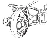
**3** Using a 13 mm wrench loosen the outside locknut (14-6). Use a 13 mm wrench to prevent the inside nut (14-3) from turning.
