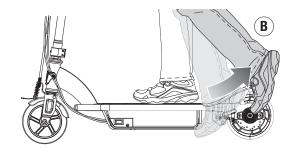
Note: Scooter must accelerate to at least 3 mph (5 kmh) for motor to engage.
