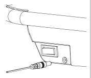
**2** Plug the charger into the charger port. Make sure the power switch is in the **OFF** position. The light on the charger should turn red during charging. The light will turn green again when charging is complete.
