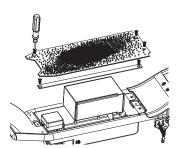
1 Using a Phillips screwdriver, remove the deck plate and lift the battery out of the tray.
