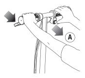
Note: As an additional safety feature, the scooter is designed to cut power to the motor when the hand brake is applied.
