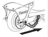
**3** With two 13mm wrenches, loosen the axle. Slide the wheel forward to loosen the chain.
