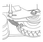
2 Using two 8mm wrenches, loosen the brake housing anchor bolts which is located in the long slot on the left side of the rear fork.
