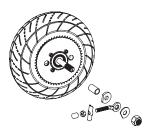
**6** Remove wheel. Note the sequence of the hardware.
