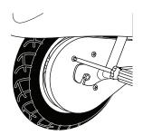
Re-attach the chain guard. Test ride and check. Readjust as needed.
