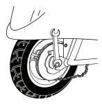
With two 17mm wrenches, loosen the axle. Push the wheel forward in the slots to loosen the chain.
