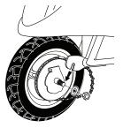
Pull the wheel out. Note the arrangement of the hardware sequence.
