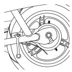
Tighten the brake housing anchor securely.
