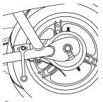
With a 10mm wrench, loosen the brake cable anchor and disconnect the cable.
