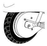
With a Phillips screwdriver, remove the screws that secure the chainguard. Remove chainguard.
