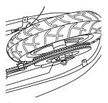
Install the new chain or wheel by slipping the chain around the axle. Slide the axle into the slots on the frame. Slide the wheel forward and maneuver the chain onto the rear sprocket, front sprocket and chain tensioner.
