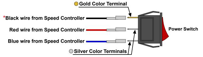
\*The black wire from the speed controller must be plugged into the gold color power switch terminal otherwise damage to the controller and other parts will occur.
