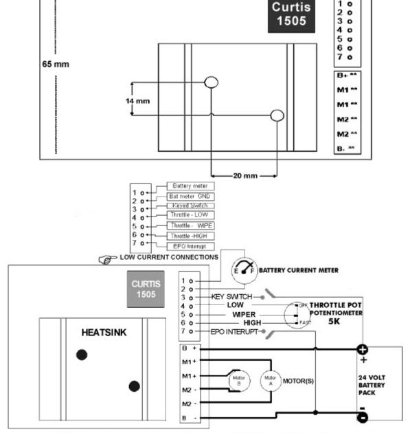
EPO Interupt = Emergency Power Off Interupt - This is typically hooked up to a brake switch to deactivate the motor when the brake is applied.
