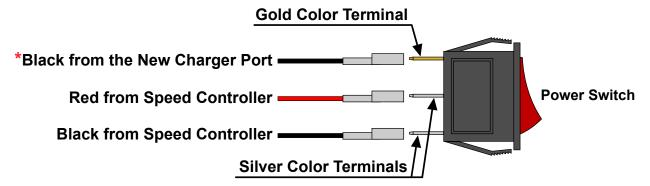
\*The black wire from the charger port must be plugged into the gold color power switch terminal otherwise damage to the controller and other parts will occur.
