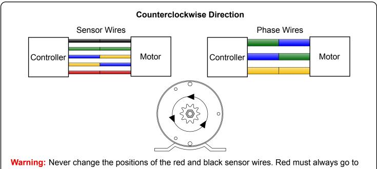
Warning: Never change the positions of the red and black sensor wires. Red must always go to red and black must always go to black otherwise damage to the motor will occur.
