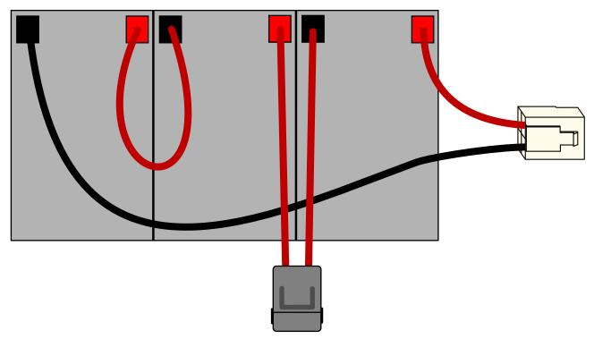
The fuse holder needs to be located on the side of the battery pack and not on top of it, otherwise it will interfere with installing the footplate.
