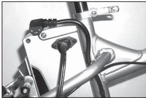
Electric Bikes with Seat Tube Mounted Battery (STB) Packs - Remove the power cable from the charger port and attach charger.
