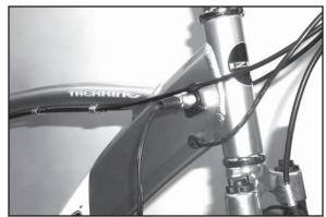
Electric Bikes with internal battery packs - Rotate the charger port cover and attach charger.
