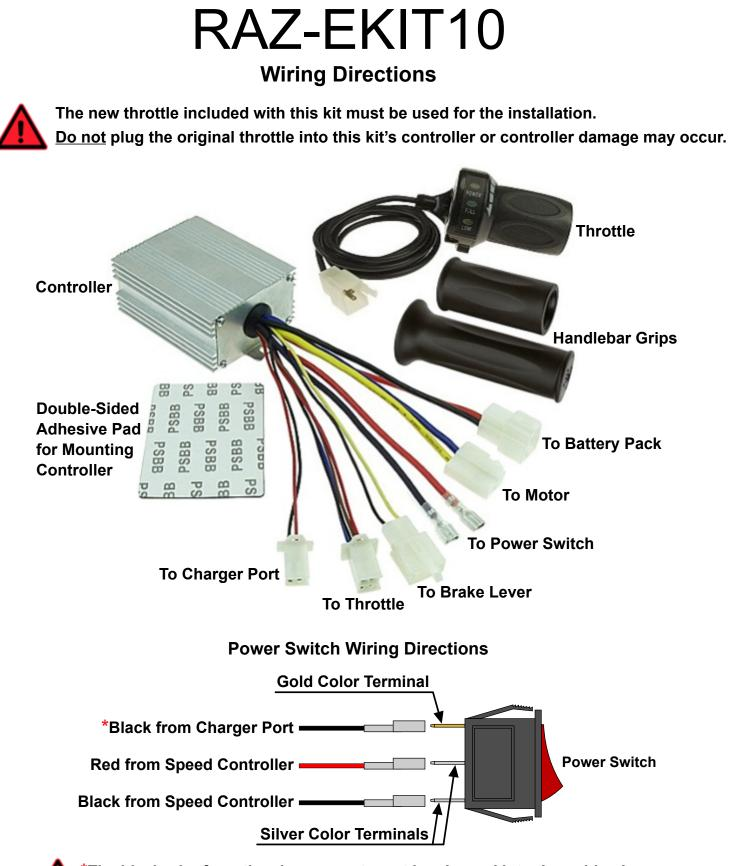
\*The black wire from the charger port must be plugged into the gold color power switch terminal otherwise damage to the controller and other parts will occur.
