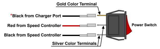
\*The black wire from the charger port must be plugged into the gold color power switch terminal otherwise damage to the controller and other parts will occur.
