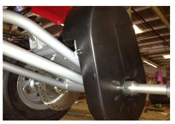
(4) remove one more screw located on the left side at the center of the chain guard, once you remove the screws you can now split open the chain guard and remove it from the unit.
