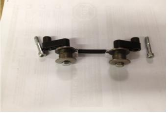
(6) Replace your chain tensioner with your new part. This a self adjusting chain tensioner and there is no need for adjustment.
