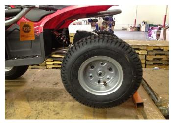
(1) To have better acces to your chain Guard you will need to remove the rear / left wheel, Using a 6mm Allen wrench loosen up and remove the 4 bolts that hold the wheel in place and pull the wheel out.
