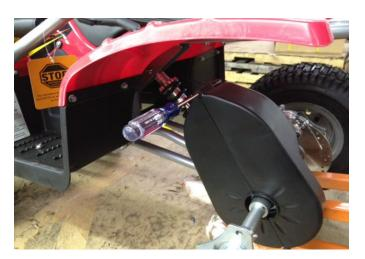
(2) Using a Philip screw driver, remove the screw on top the chain guard
