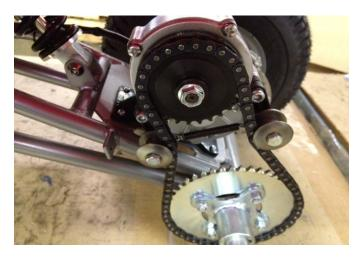
(5) Using a 5mm Allen wrench remove the two bolts that hold the chain tensioner onto the motor and remove it.
