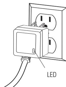
**1** Plug the charger plug into wall outlet. The light on the charger should be green.
