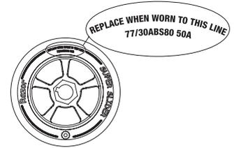
**Note:** The Ground Force Drifter Fury wheels must be replaced when worn down to the wear indicator line.
