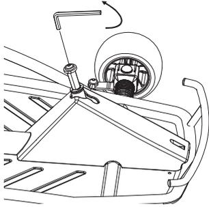
**1** Using a 5 mm Allen wrench, loosen the screw located in the steering column.
