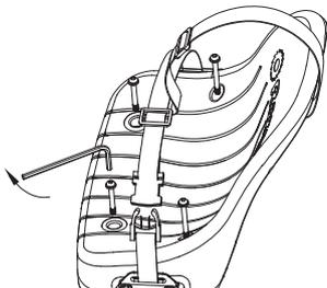
**1** Using a 5 mm Allen wrench, loosen the four (4) seat bolts and remove seat.
