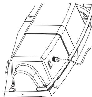
**2** Make sure the power switch is in the **OFF** position. Plug the charger into the charger port on the Ground Force Drifter Fury. The light on the charger should turn red during charging. The light will turn green again when charging is complete.
