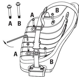
**1** Position the seat over the frame and align it with the holes in the frame. Align the safety belt anchor holes to the holes in the seat and frame with the lap/shoulder assembly on the left and the receiver latch on the right. Insert the four (4) seat bolts and tighten securely.
