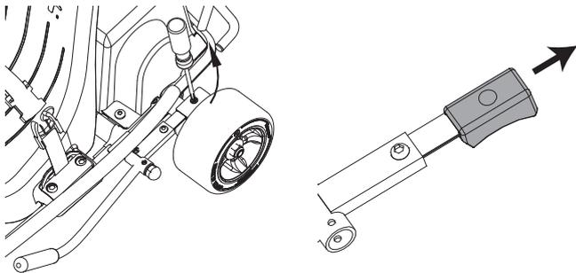
**1** Using a Phillips screwdriver, loosen the screw on the spark cartridge and remove the cartridge.
