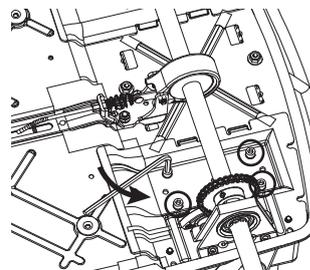
**6** Using a 5 mm Allen wrench, loosen the four (4) bolts holding the motor to the frame. Carefully lower the motor and remove chain from around the motor sprocket.
