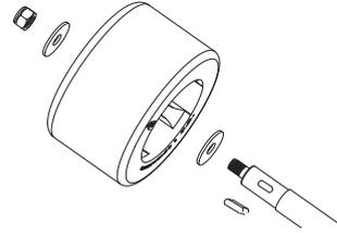
**3 Rear Wheel Installation:** Make sure the key way is properly seated in the rear axle and aligned with the key way in the wheel. Position the wheel with the **Razor logo facing outward**. Install the washer and tighten the self-locking nut securely.
