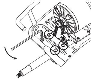
**3** Remove the eight (8) bolts (four on each side) that attach the brackets to the frame.
