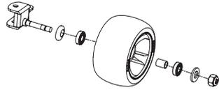
**2 Front Wheel Installation:** Make sure the bearings are properly seated and the center spacer is installed. Position the wheel with the **Razor logo facing outward**. Install the washer and tighten the self-locking nut securely.
