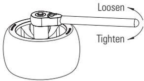
**1 Removal:** To remove a wheel, remove the self-locking nut. Tap the wheel to remove.
