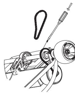
**3** Using a flat head screwdriver, carefully re-attach the clip on to the link plate. The clip must point in the drive direction of chain rotation.
