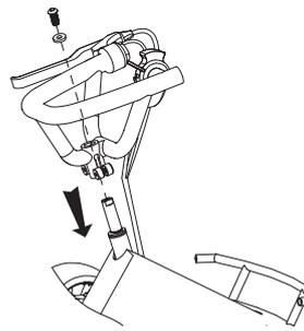
**2** Make sure the wires are not tangled. Insert the steering wheel, washer and screw into the steering column as shown.
