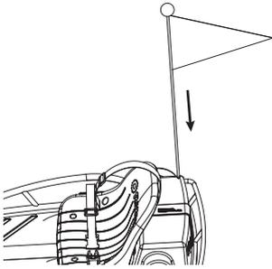
**1** Locate the hole located on the top right side of the battery cover. Insert the flag.
