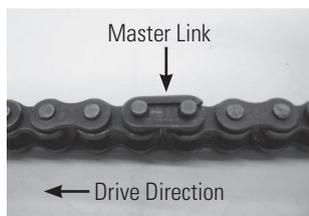
**1** Locate the master link on the replacement chain and with a flat head screwdriver carefully disengage the clip from the chain to remove the link plate and connector link.
