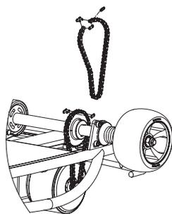
**2** Wrap the chain around both sprockets and tension idler. Insert the connector link all the way through the chain and fit the link plate over the connector link.
