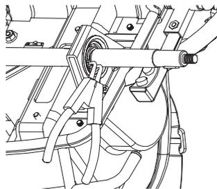
**8** Remove the two (2) "C" clips (one on each side). Remove the two (2) brackets that hold the rear axle in place and remove axle.
