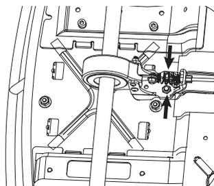
**4** Carefully turn unit over and loosen the two (2) bolts next to the brake cable.
