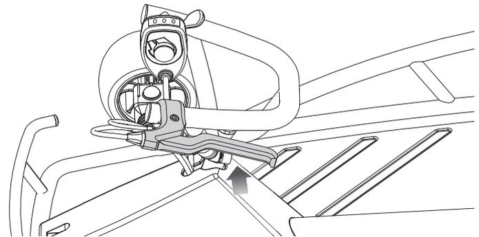
To activate the sparking feature, pull up on the Spark Bar handle (no more than 5 seconds at a time), then release. Allow 20 seconds between sparks to prevent overheating the spark components.
