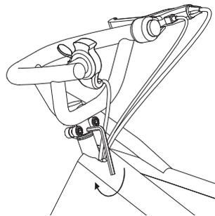
**4** Using a 5 mm Allen wrench, alternately tighten each of the bolts on the steering wheel clamp. When the bolts are properly tightened, the gap between the clamp halves should be even.
