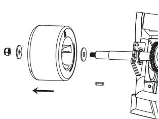
**7** Using a 17 mm wrench, loosen the lock nut on both rear wheels and remove wheels. If necessary, gently tap rear wheel with a rubber mallet to help loosen wheel off the rear axle.
