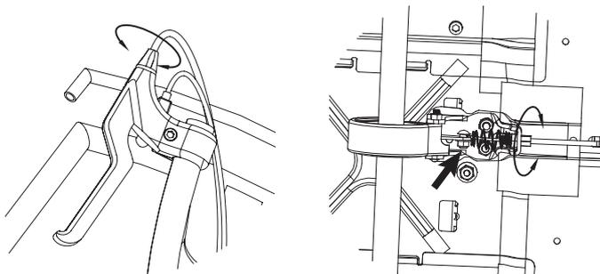
**1** To adjust the brake, thread the adjuster in or out 1/4 to 1/2 turns until the desired brake adjustment is attained.
