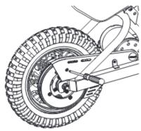
**1** Loosen screw and remove chain guard.
