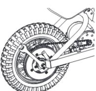
**2** Using two 19mm wrenches, loosen both axle nuts.
