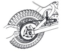
**4** Install the new chain or wheel by slipping the chain around the axle. Slide the axle into the slots on the frame. Slide the chain tensioner down and maneuver the chain onto the rear sprocket and front sprocket.
