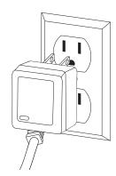
1 Plug the charger into a wall outlet. If the lights on charger do not light up, check the power to the outlet. If necessary, try a different outlet.
