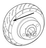
**6** Remove wheel and replace chain or tire. To reinstall wheel, reverse these steps.
