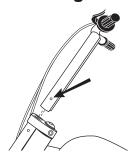
**1** Press the spring buttons on each side of the handlebars and tap the bars until the spring buttons slide inside and engage the corresponding holes in the fork
