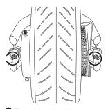
3 Tightening the adjusters clockwise tightens the chain; loosening the adjusters counterclockwise will relax it. When loosening the adjusters, you will have to nudge the axle forward by tapping the wheel with your hand to relax the tension on the chain.
