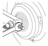
**4** Turn both adjusters the exact same amount, 1/8 to 1/4 turn at a time, to maintain the wheel alignment. Once the tension is correct, tighten the axle and brake anchor bolt.
