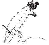
**2** When correctly engaged, the handlebars will not disengage from the fork.
