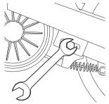
**2** Loosen and disconnect the brake housing anchor. Note: Pay attention to the location of the parts for when you reinstall.
