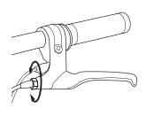
1 To adjust the play, thread the brake lever adjuster in or out 1/4 to 1/2 turn until the desired brake adjustment is attained. Most adjustments are complete at this step. If brake still needs further adjustment, proceed to step 2.
