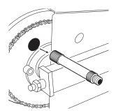
**3** Remove valve adapter immediately after inflating.
