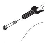
**1** Use the special valve extender/adapter supplied. This item is concealed in the grip on the speed control side of the handlebar.
