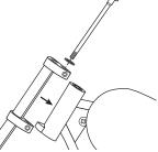
2 Slide the fork into position and insert the steering bolt. The bolt must go through the washer and spacer sleeve and between the steering bearings inside the frame.
