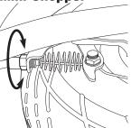
**2** If the brake lever adjuster is threaded outward and the brake still has too much slack, use the rear brake adjuster for additional adjustment.
