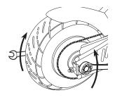
**3** Loosen the rear axle by attaching wrenches to both axle nuts and loosening counterclockwise.
