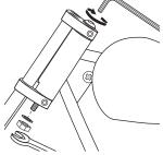
**3** Install washer and nut onto steering bolt. Tighten until snug, then back off slightly to allow the steering to rotate freely with no binding or end-play.
