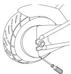
1 Loosen screw and remove chain guard.
