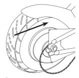
**3** Slide the wheel forward to slacken the chain and disengage the chain from the wheel sprocket and motor sprocket.
