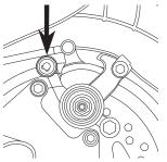
**3** If the brake rotor is dragging on the brake pads use your fingers to twist the calliper adjuster in either direction until rotor is centered between pads.
