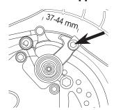
2 If the brake has too much slack, loosen the rear anchor bolt and pull the brake wire tighter. The distance of the brake wire between the end of the cable and the anchor bolt should be between 37-44 mm.
