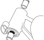
**1** Insert the spacer sleeves on the top and bottom of the frame.
