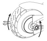
**2** Loosen the rear axle by attaching wrenches to both axle nuts and loosening counterclockwise.
