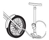
**1** Using a bicycle style tire pump equipped for a Schrader-type valve, inflate the front tire to the PSI indicated on the sidewall of the tire.
