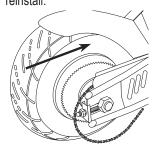
**5** Slide the wheel forward to slacken and disengage the chain from the wheel sprocket and motor sprocket.
