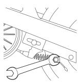
**1** Loosen and disconnect the brake cable anchor.
