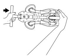
Fold the front wheel stem down and push inward and down to snap it into the clamp.
