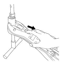
Stick your finger in the circular lever and pull back to unlock and release front wheel stem
