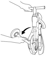
Grasp the handle bar and the pull lever on the stem of the rear wheel. Pull the hand grip toward the wheel to release from the locked position. Pull outward until it snaps into place. Repeat for other rear wheel.
