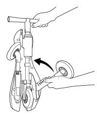
Grasp the hand grip on the stem of the rear wheel. Pull the hand grip toward the wheel to release from locked position. Fold inward until it snaps into place. Repeat for other rear wheel.
