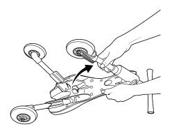
Grasp the front wheel stem and pull out to release from clasp. Pull forward until you hear it snap into place.
