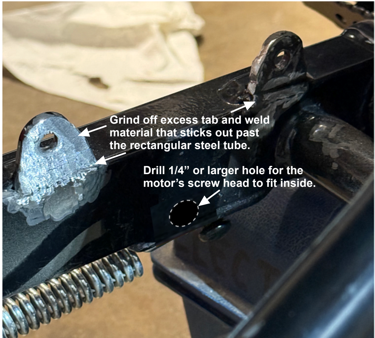
Photo of corrections made to the swing arm so the back of the motor fits flush to the swing arm.
