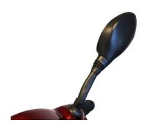
To attach the mirror simply place each mirror threaded end into the mirror post. Turn mirror clockwise and fasten mirror to scooter.
