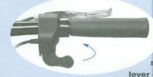
To start and accelerate your Lashout™, simply press the lever of the throttle. As
