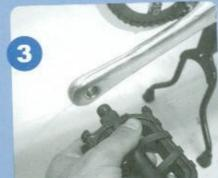
Turn the left pedal axle counter-clockwise until tight.
