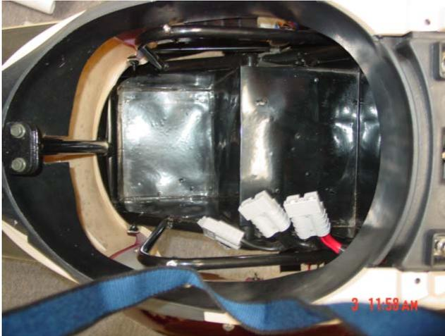
3. Place the battery with the longest cable into the battery compartment. The cable measures 18 ½" in length (The measurements are taken from the base of the black cable to the top of the connector). Make sure the cable set aside so that you will be able to connect it.
