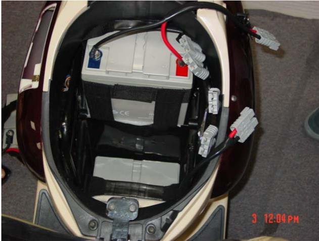
5. The next battery that you want to install goes on top of the battery on the bottom, this cable 14" in length (The measurements are taken from the base of the black cable to the top of the connector). Make sure the cable set aside so that you will be able to connect it.
