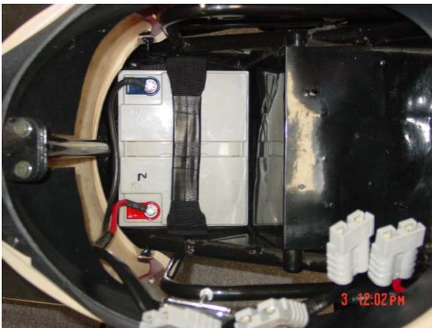
4. The next battery that you want to install goes on the second tier. This is the shortest cable 11" in length (The measurements are taken from the base of the black cable to the top of the connector). Make sure the cable set aside so that you will be able to connect it.
