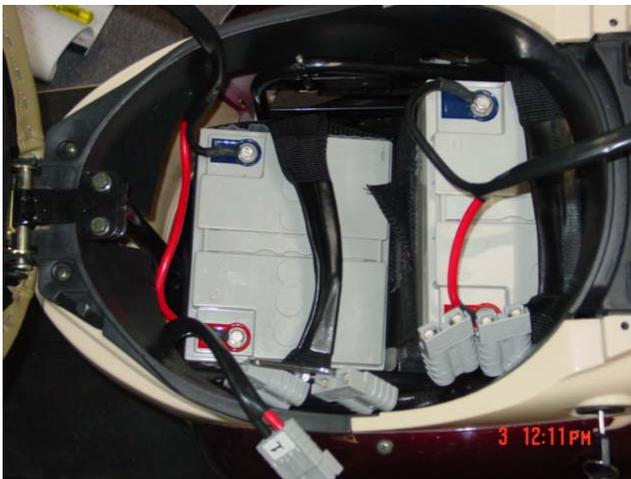
6. The next step is to place the remaining battery on top of the previously installed one, this cable 14" in length (The measurements are taken from the base of the black cable to the top of the connector). Make sure the cable set aside so that you will be able to connect it.
