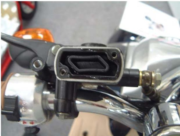
5. Add brake fluid, DOT 3 or DOT 4, fill above the line on the outside of Brake Fluid window.
