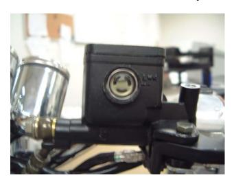
2. Remove the screws on outer cover.
