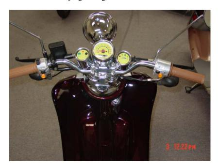
4. Clean and adjust both mirrors before you ride. Adjust each mirror so you can see the lane behind you and as much as possible of the lane next to you. When the mirror is properly adjusted you can see the edge of your arm and shoulder.
