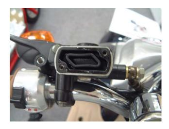
5. Add brake fluid, DOT 3 or DOT 4, fill above the line on the outside of Brake Fluid window.
