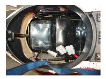
3. Place the battery with the longest cable into the battery compartment. The cable measures  $18\frac{1}{2}$  "in length (The measurements are taken from the base of the black cable to the top of the connector). Make sure the cable set aside so that you will be able to connect it.
