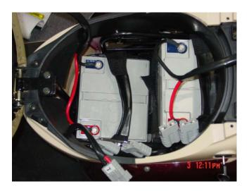
6. The next step is to place the remaining battery on top of the previously installed one, this cable 14" in length (The measurements are taken from the base of the black cable to the top of the connector). Make sure the cable set aside so that you will be able to connect it.
