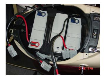
7. Once you have placed all of the batteries into the compartment you must connect the batteries to the female plugs.
