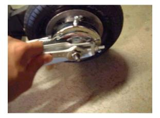
Step 3.) Remove the axle nut located on the right side of the rear tire as seen in Fig 3.
