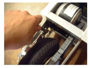
Step 2) Remove screw holding brake shield in place (see fig. 2) located next to the left side of the rear tire. This bolt connects the brake shield to the frame.
