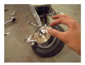
Step 7.) Place the brake shield back on the wheel's slide axle brake into the tire and remember to place the pacer between the brake shield and brake drum.
