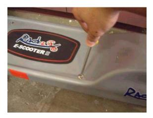
Step 1) Remove the 3 screws from the deck, use the Medium size Allen wrench to remove screws as shown in Figure 1. Lift the deck.
