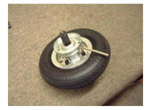
Step 6.) Remove the Allen bolts from the rim of the tire; you must first cut ½" off of the medium size Allen wrench (use hack saw). The rim will split into 2 pieces. Once apart, replace the old tire with the brand new tire you have just received. Reassemble the rim back onto the tire.
