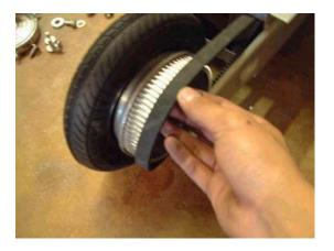
Step 8.) Next place the wheel hub back into the rear fork and reinstall the drive belt. Retighten the axle bolts.
