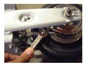
Step 4.) Loosen the brake adjustment bolt as seen in Fig 4. Do not completely remove this bolt. It should loosen to the point where the line traveling through the "brake spring" can be removed. Next remove the drive belt from the tire sprocket. Once this has been completed, the rear tire and hub can be removed from the scooter.
