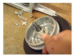
Step 5.) Remove the axle bolt from the rear wheel; take not of where the spacers are located.
