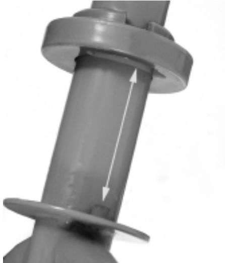
Figure 2. Steering bushing and fork. Align the slot with the peg (arrow).
