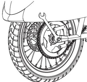
**2** Using two (2) 15 mm wrenches, loosen the locknuts. Slide the wheel forward to loosen the chain and remove the wheel.
