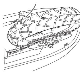
**3** Install the new chain or wheel by slipping the chain around the axle. Slide the wheel forward and maneuver the chain onto the rear sprocket, motor sprocket and chain tensioner.
