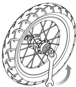
**1** Using two (2) 15 mm wrenches, remove the locknuts and lock washers on both sides of the front wheel, then remove front wheel.
