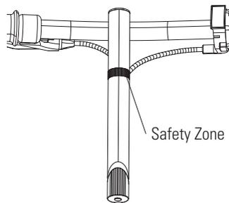
**5** Slowly slide the handlebars up to make certain that the bar is in the "SAFETY ZONE". Failure to secure the handlebars within the safety zone can cause the handlebars to come out while riding.
