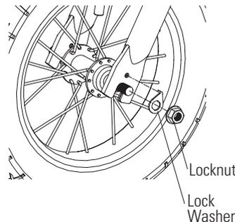
**3** Insert the tab on the lock washer into the hole on the front fork and tighten the 15 mm locknuts on both sides of the wheel.
