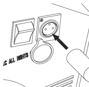
**2** Make sure the power switch is in the **OFF** position. Plug the charger into the charger port on the product. The light on the charger should turn red during charging. The light will turn green when charging is complete.
