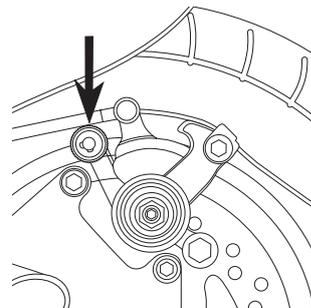
**3** If the disc brake is dragging on the brake pads, use your fingers to twist the caliper adjuster in either direction until disc is centered between pads.
