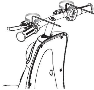
**2** When desired position is reached, re-tighten bolt until brake levers are securely in place.
