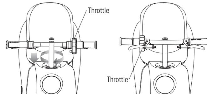
**4** While inserting the steering tube down into the handlebar tube, hold steering bolt steady with thumb and rotate handlebars 180 degrees to the left.
