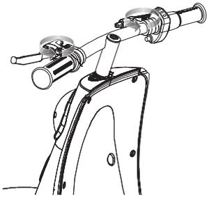
**1** Loosen the 5 mm bolt located on the brake levers to adjust the angle of the brake levers to a comfortable position for the rider.
