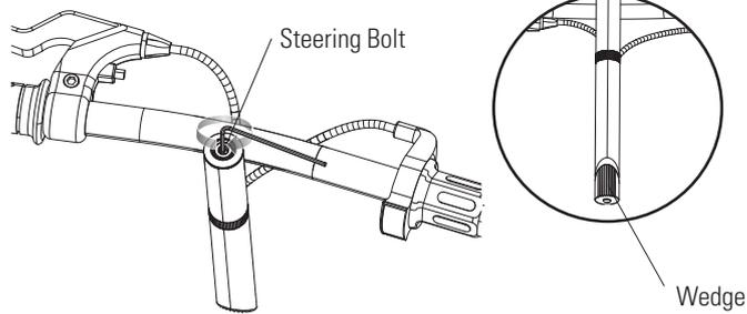
**2** Using a 6 mm Allen wrench, loosen steering bolt in four (4) complete turns so that the wedge is loose and not touching steering tube.
