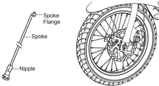
**1** Verify spoke tension by grasping and shaking each spoke. Spoke should not be loose from hub. Look for any play between spoke flanges where it mates with hub. Try to turn nipple using your fingers. You should not be able to spin any nipple by hand. If one or more spokes are loose, or if you can turn any nipple using your fingers, all spokes must be checked and need to be tightened with a spoke tightener.
