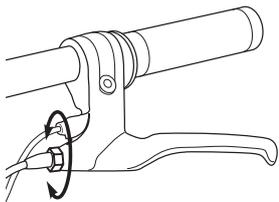
**1** To adjust brake cable play, thread the brake lever adjuster in or out 1/4 to 1/2 turn until the desired brake adjustment is attained. Most adjustments are complete at this step. If brakes still needs further adjustment, proceed to step 2.
