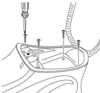
**1** Open up seat and loosen the four (4) Phillips screws located inside the storage compartment and remove tray.
