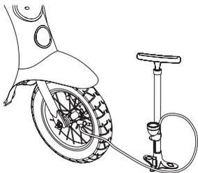
Using a bicycle tire pump equipped for a Schrader valve, inflate the tires to the PSI indicated on the sidewall of the tires.
