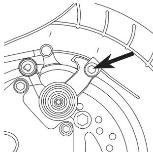
**2** If the brake has too much slack, loosen the rear anchor bolt with a 5 mm Allen wrench and pull the brake wire tighter. The distance of the brake wire between the end of the cable and the anchor bolt should be between 37 mm and 44 mm.
