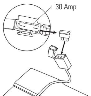
**3** Remove the fuse and replace with a new one of equal amperage. Close fuse box. Reattach storage compartment.
