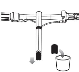
**1** Remove plastic protector at the end of the steering tube.
