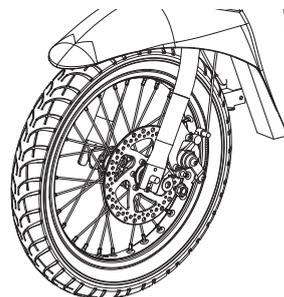
**3** Re-insert the tab on the lock washers into the holes on the front fork and tighten the locknuts on both sides of the wheel.
