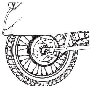
**4** Verify chain is properly installed on each sprocket and chain tensioner is correctly positioned at the bottom of the chain.
