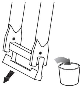
**1** Remove the plastic packing material from the front fork.
