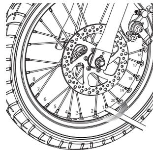
**2** Start with spoke closest to tire valve and tighten each nipple. In sequence, exactly 1/4 to 1/2 turn. A single 1/4 to 1/2 turn may not be enough to bring the spokes into proper tension. Continue tightening all spokes in sequence, no more than 1/2 turn until all spokes are tight.
