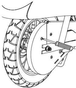
**1** Loosen the five (5) Phillips screws on the chain guard. Remove chain guard.
