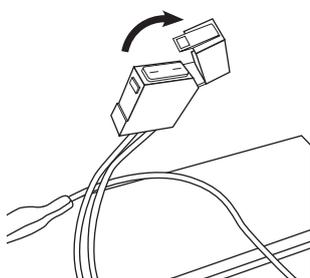
**2** Locate fuse box on top of batteries. Open the fuse cover to expose the fuse.
