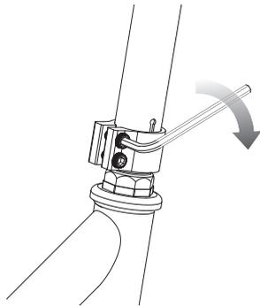
**2** With the front wheel pointed straight ahead and the handlebars square to the front wheel, tighten both bolts on the clamp with a 5 mm Allen wrench. Tighten securely.
