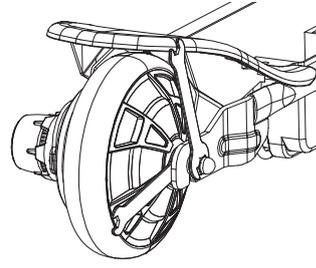
**3** Using a 13 mm wrench loosen the outside locknut (14-6). Use a 13 mm wrench to prevent the inside nut (14-3) from turning.
