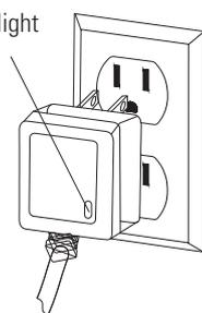
**1** Plug the charger plug into wall outlet. The light on the charger should be green.
