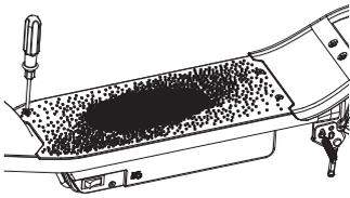
**7** Using a Phillips screwdriver reinstall deck plate.
