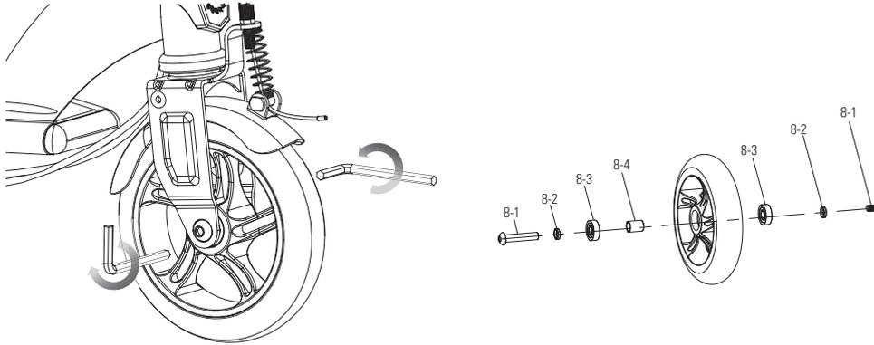
**1** Using two (2) 5 mm Allen wrenches, loosen the axle bolt. Remove wheel and install replacement wheel. (Note the sequence of the hardware)
