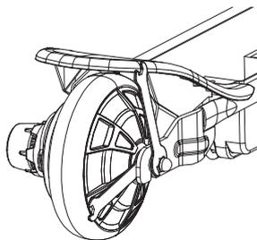
**5** To reinstall the wheel/motor, reverse steps 4 through 1, taking care to use a wrench to hold the inside locking nut, while tightening the outside axle nut (shown).
