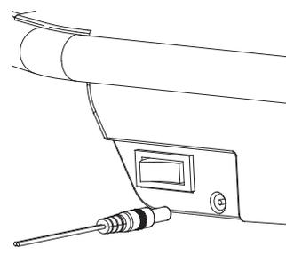
**2** Plug the charger into the charger port. Make sure the power switch is in the **OFF** position. The light on the charger should turn red during charging. The light will turn green again when charging is complete.
