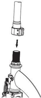
**1** Loosen the collar clamp. With a side to side twisting motion, push and twist to slide the handlebar onto the fork until it bottoms out on the headset locknut.
