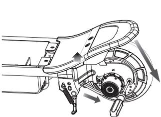
**4** Using a Phillips screwdriver, remove the two (2) screws that attach the motor housing to the frame.
