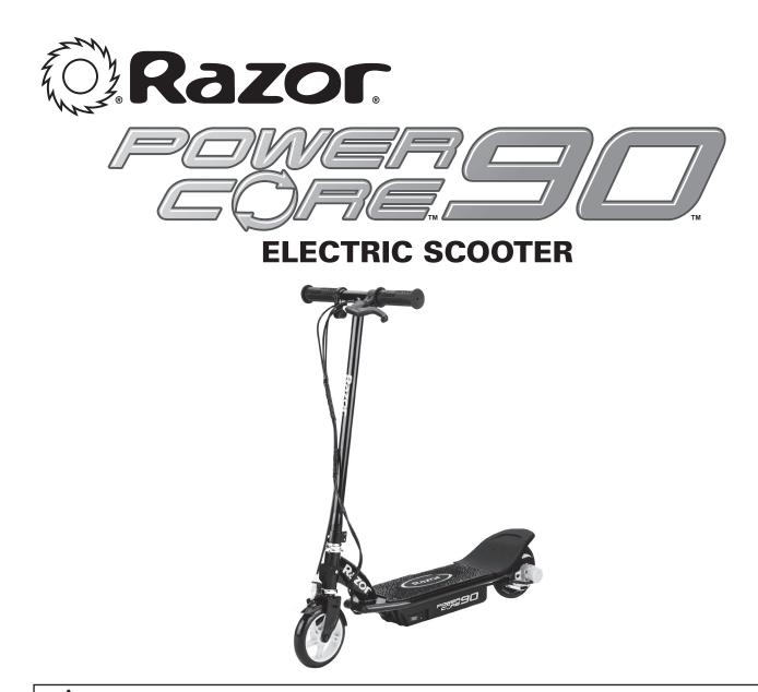
**NOTE:** The unit must be traveling at least 3 mph (5 kmh) before motor will engage. Kick start to at least 3 mph (5 kmh) while applying the push button throttle to engage motor.
