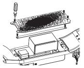
1 Using a Phillips screwdriver, remove the deck plate and lift the battery out of the tray.
