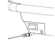
**2** Plug the charger into the charger port. Make sure the power switch is in the **OFF** position. The light on the charger should turn red during charging. The light will turn green again when charging is complete.
