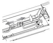
2 Using a Phillips screwdriver, remove the cable-clamping block and disconnect the motor connector from the controller.
