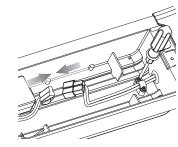
6 Reconnect the motor connector, reinstall the cable clamping block (shown), and reposition the battery and replace cover, tighten cover screws.
