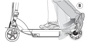
Note: Scooter must accelerate to at least 3 mph (5 kmh) for motor to engage.
