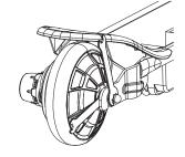
**5** To reinstall the wheel/motor, reverse steps 4 through 1, taking care to use a wrench to hold the inside locking nut, while tightening the outside axle nut (shown).
