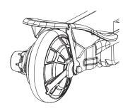
**3** Using a 13 mm wrench loosen the outside locknut (14-6). Use a 13 mm wrench to prevent the inside nut (14-3) from turning.
