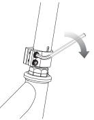
**1** Loosen the collar clamp. With a side to side twisting motion, push and twist to slide the handlebar onto the fork until it bottoms out on the headset locknut.
