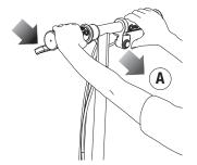
**Note:** As an additional safety feature, the scooter is designed to cut power to the motor when the hand brake is applied.
