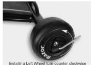
using a wrench, tighten both locknuts against the frame. If the wheel will not spin freely, loosen the locknuts and unthread the axle about 1/4 turn and adjust the locking nuts in or out until the wheel spins free with little or no side play. The correct adjustment is where the wheel spins free, has the least amount of endplay as possible, and both lock nuts are tightened securely against the frame.
