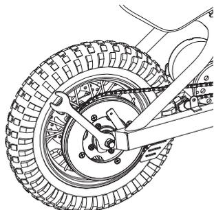
**2** Using two 19 mm wrenches, loosen both axle nuts.
