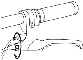
**1** To adjust brake cable play, thread the brake lever adjuster in or out 1/4 to 1/2 turn until the desired brake adjustment is attained. Most adjustments are complete at this step. If brake still needs further adjustment, proceed to step 2.
