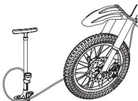
**1** Using a bicycle-style tire pump equipped for a Schrader-type valve, inflate the front tire to the correct PSI indicated on the sidewall of the tire.
