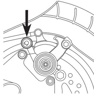
**3** If the brake rotor is dragging on the brake pads, use your fingers to twist the caliper adjuster in either direction until rotor is centered between pads.
