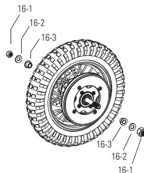
**Note:** the arrangement of the hardware sequence:
