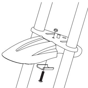
**1** Align fender with the hole in the fork and insert the bolt. Tighten securely using a 10 mm wrench and 5 mm Allen wrench.
