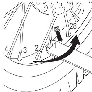
**1** Verify the spoke tension by shaking each spoke with your fingers. Spoke should not be loose from hub. Look for any play between where the spoke flanges attach to the hub. Try to turn the nipple using your fingers. You should not be able to spin any nipple by hand. If one or more spokes is loose, all spokes must be checked and need to be tightened with a spoke wrench.
