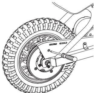
**1** Loosen screws and remove chain guard.
