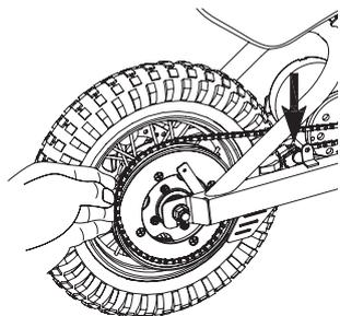
**4** Install the new chain or wheel by slipping the chain around the axle. Slide the axle into the slots on the frame. Slide the chain tensioner down and maneuver the chain onto the rear sprocket and motor sprocket.
