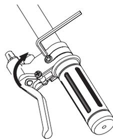
**3** Adjust the brake lever adjuster to the proper place and tighten it with the 5 mm Allen wrench.
