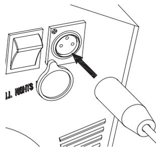
**2** Make sure power switch is in the **OFF** position. Plug the charger into the charger port. The light on the charger should turn red during charging then back to green when charging is complete.
