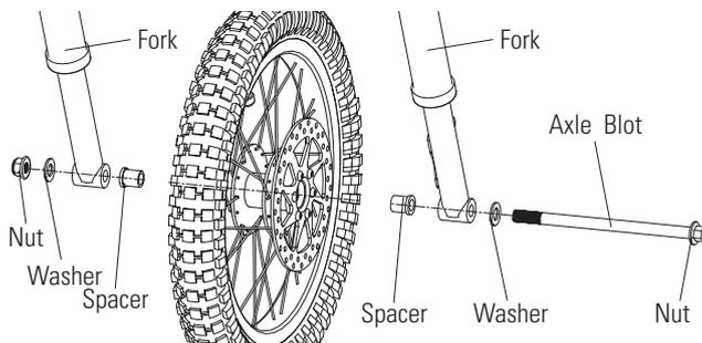
**2** Slide axle through fork, spacer and wheel hub. When axle passes through the other side of the wheel hub, add the other spacer, and slide through the fork. Secure with washer and nut.
