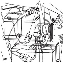
**1** Remove the seat fairing and battery cover to locate the 3 fuse boxes attached to the batteries.
