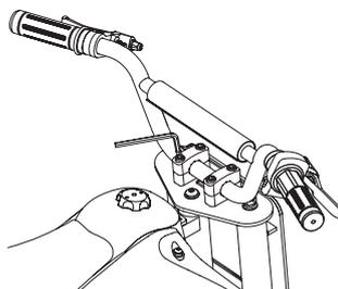
**2** Align parallel to the fork and tighten the bolts using a 6 mm Allen wrench. When properly tightened, the handlebars should not move forward or backward.
