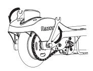
**2** Using two 13mm open wrenches, loosen the locknuts by turning the wrenches counter clockwise.
