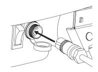
**2** Turn power **OFF** before charging. Plug the charger into the charger port on the electric scooter.
