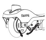
**3** To loosen the chain, push the chain tensioner down to create some slack in the chain.
