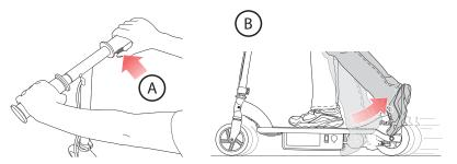
To start unit, turn on power switch, press the push button throttle (A) and kick start up to 3mph (5mh) (B).
