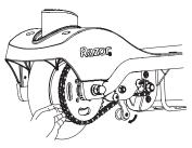
**5** Push the chain tensioner down to install the chain on both sprockets.
