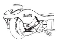
**1** With a Phillips screwdriver, loosen the two screws and remove the chain guard.
