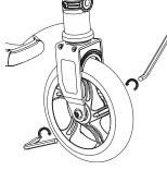
**1** Using two (2) 5mm Allen wrenches, loosen the axle bolt. Remove wheel and install replacement wheel. (Note the sequence of the hardware)
