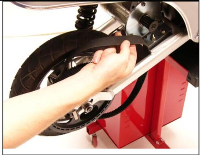
3. Install the rear wheel onto the scooter frame.
