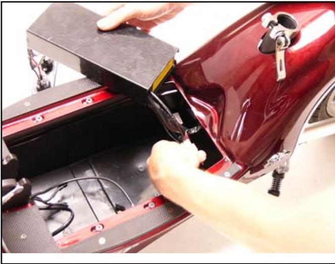
7. Unplug the three larger connectors at the back of the controller.
