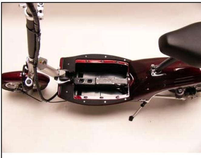
1. Turn the scooter power off and remove both batteries.
