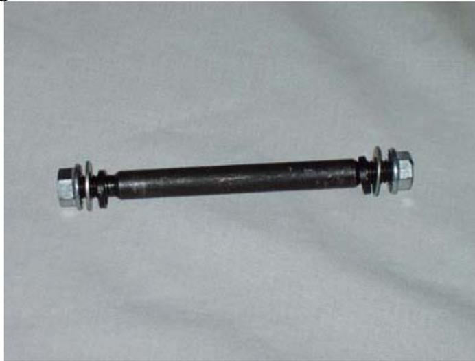
Remove the nuts and washers and insert the axel into the wheel. The black washer goes in between the wheel and fork while the flat washer goes on the outside of the fork and then is secured in place with the nut.
